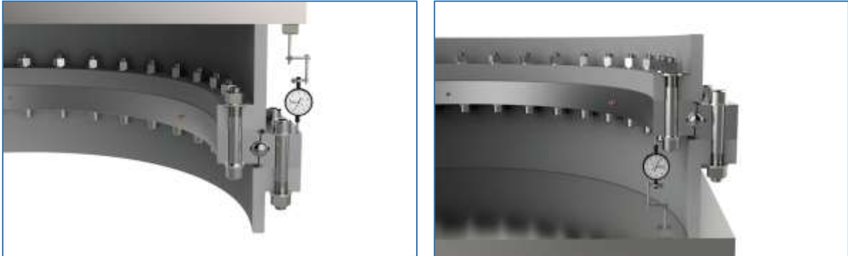
Figure 4.8. – Measuring of the tilting/axial clearance
