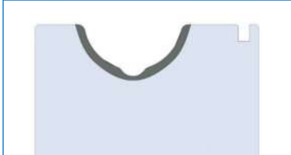
Figure 2.8. – Ball bearing raceway hardened layer
