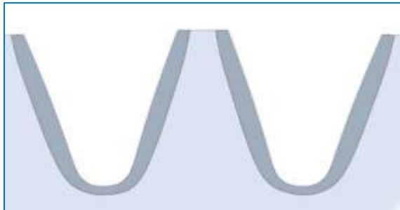
Figure 2.10. – Gear gap hardening
